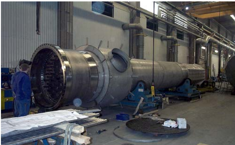
Figure 8: Fabrication of the HTCR tube bundle
