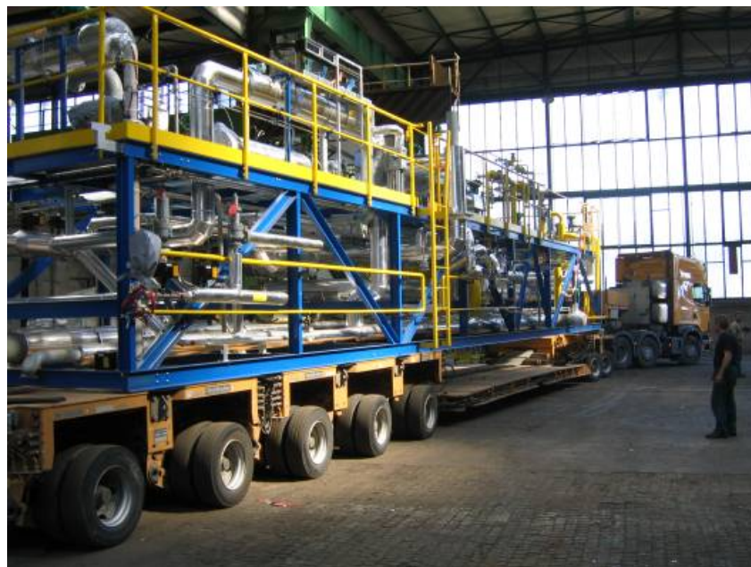
Figure 9: Transportation of skids from workshop
