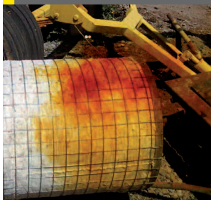
Fig 1: NO x emission from candle filter during cleaning
