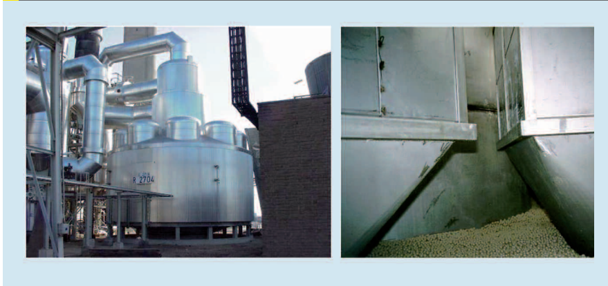
Fig 4: The single-bed SO 2 converter with risers holding the DeNOx catalyst at Nyrstar Budel Zink, The Netherlands
