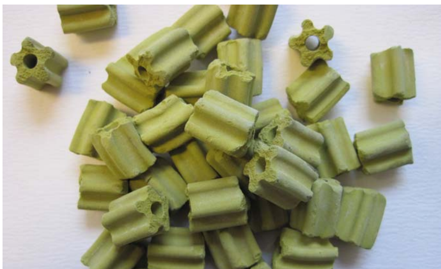
Figure 2. The new VK-701 LEAP5™ catalyst in 12 mm Daisy shape.
