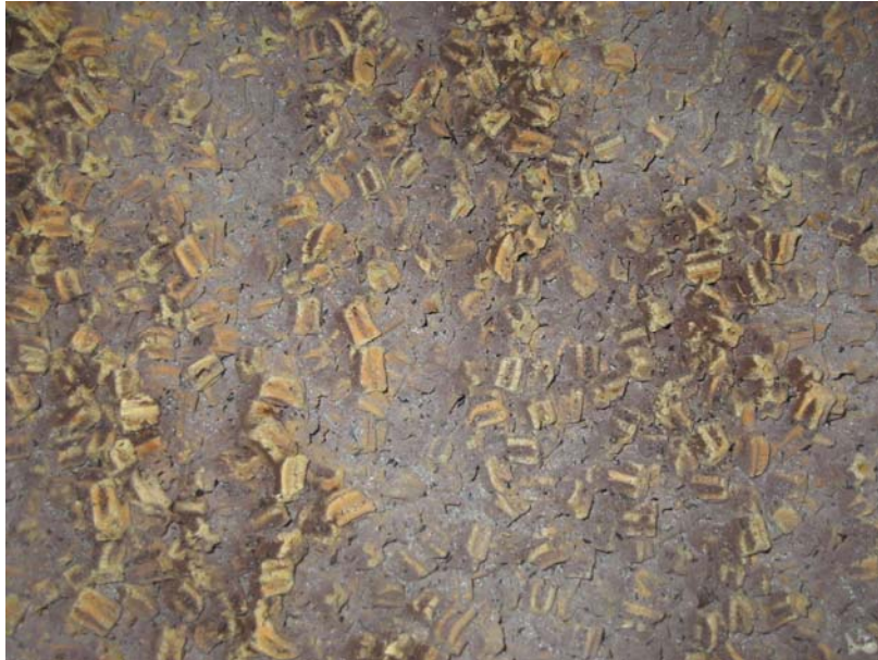
Dust deposited in a 1 st bed loaded with Topsøe 12 mm Daisy catalyst.
