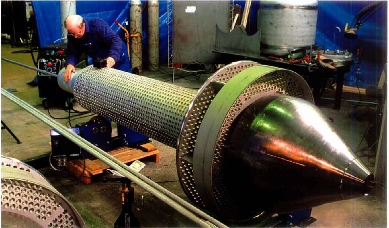
Topsøe CTS Burner for an oxygen-blown autothermal reformer
