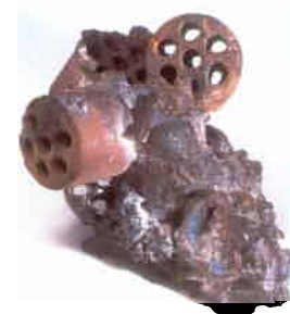
Figure 1: Melted burner tip with undamaged secondary reforming catalyst RKS-2-7H
