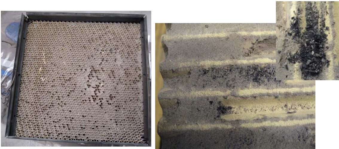
Figure 11 Severe plugging of the SCR catalyst Studstrup Power Station's Unit 4 caused by large straw-ash particles, seen as black particles in the otherwise grey coal ash
