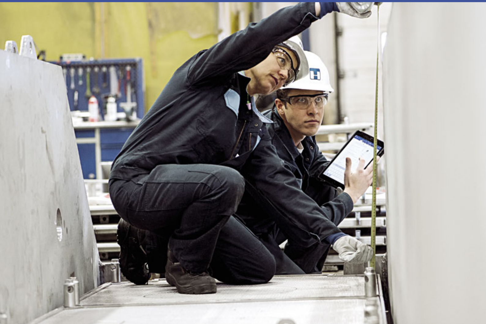
Reactor internals are inspected before shipment.
