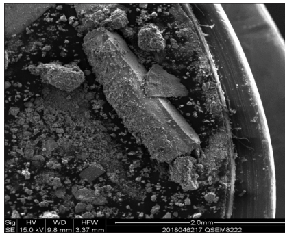
Figure 5 Millimetre-sized debris from steel degradation due to corrosion and/or erosion particles downstream of the feed filter
